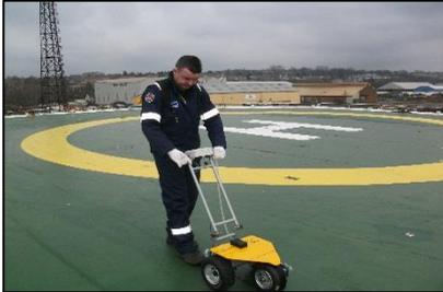
Findlay Irvine are world leading experts in measuring skid resistance for airports having been manufacturing Continuous Friction Measuring Equipment (CFME) for over 20 years. Currently in use in over 550 airports worldwide, GripTester MK2 is the world's most versatile, robust and deployable continuous friction measuring device. Also now available is the micro GripTester for Helidecks.
